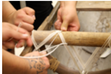
Image: Constructing the Pa'u lashing design using rope to connect the 'iako (boom) to the wae (spreader) in the wa'a.
